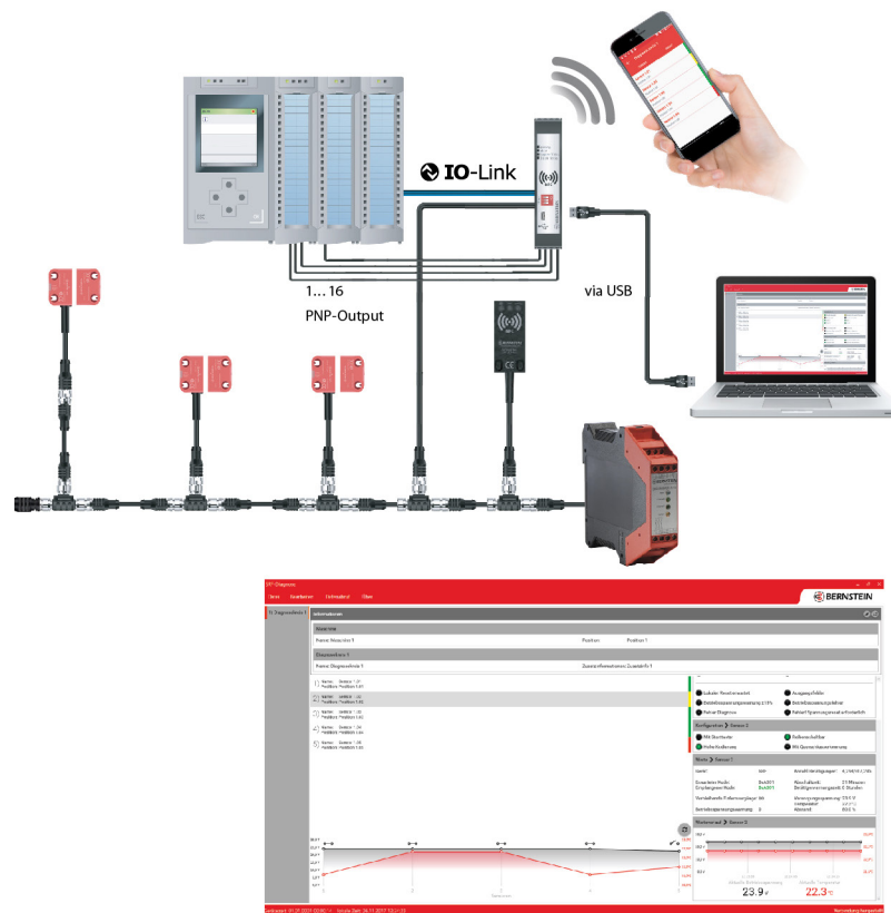
Figure 6: Safety diagnostics operate independently of the safety outputs.
