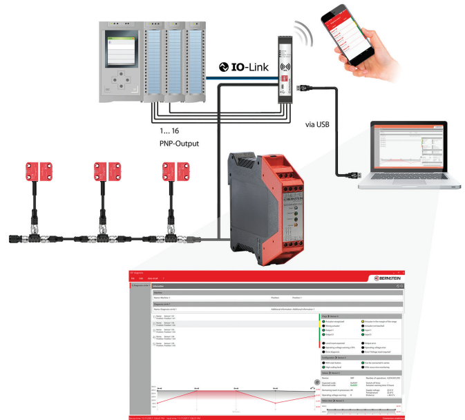
FIGURE 3: One of the more important options the SRF Safety Sensor provides is full diagnostics for better control and analysis of the system.
