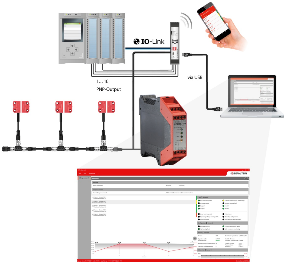
Figure 3: Daisy Chain Diagnostics make the machines more efficient and enable predictive maintenance to be realized. Source: Bernstein AG
