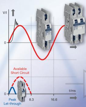
Current limiting circuit breakers minimizes the short circuit current to a relatively small amount in an extremely short time. This limits the short circuit potential harmful energy.
