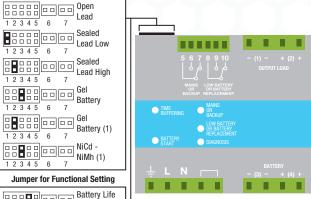
Jumper present: fast test enabled.
