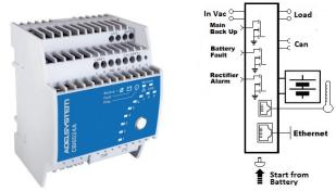
Power Management: Thanks to the All In One units (DC-UPS), it will be possible to optimize power management. The available power is automatically allocated between load and battery, supplying power to the load is the first priority of the unit thus it is not necessary to double the power, because also the power going to the battery will go to the load if the load so requires. The maximum available current on the load output is 3 times the value of the device rated current In.
