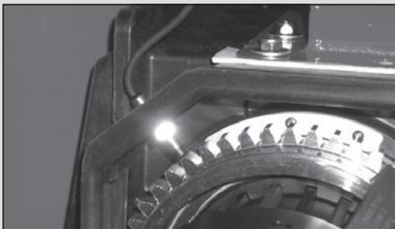
The fact that many non-magnetic metals allow magnetic fields to pass unhindered also extends the fields of application for magnetic sensors. This makes it possible to encapsulate sensors in a sturdy pressure-proof metal enclosure. Sensors can, however, also be mounted in tubing or concealed behind non-magnetic metal surfaces.
