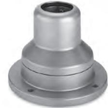
Rotary wall coupling for directly mounting on vertical machine surfaces. Angle of rotation 340° with limit stop. Cover for easy cable installation. Preset torque. Maintenance-free bearings. Complete with seals and mounting material
