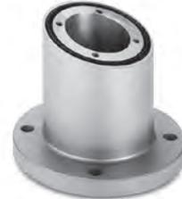
Rotary base coupling (external mounting) for directly mounting enclosures on machines or floors. Angle of rotation 340° with limit stop. Preset torque. Maintenance-free bearings. Complete with seals and mounting material
