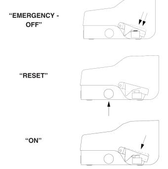
**Step 3:** In an emergency, if the pedal is depressed beyond the pressure point, the machine will stop. Beyond the pressure point, the contacts are locked in the "OFF" - Position. The machine cannot operate at this time.
