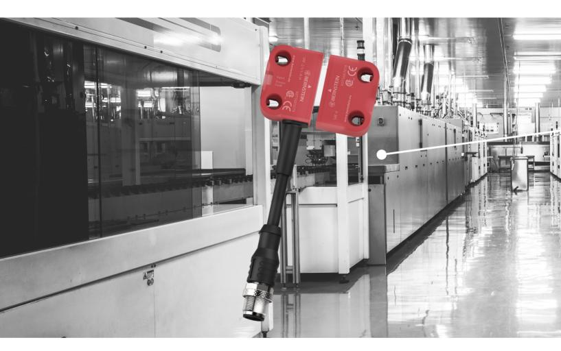
The SRF (Safety RFID) is a non-contact safety sensor, that monitors moveable safety guards, such as doors, flaps and hoods. This particularly compact sensor protects employees from injuries by shutting down or not starting up machines when the safety guard is not properly closed.
