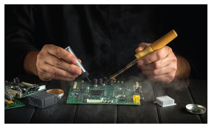
*Figure 8:* Besides automated soldering solutions, manual soldering if often necessary when a PCB component needs to be replaced.
