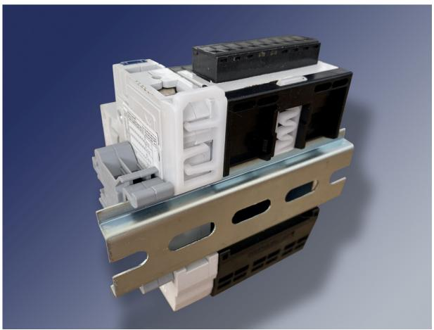
Figure 2. A rear view of a DIN rail with a two-pole circuit breaker mounted on it. The circuit breaker is displayed upside-down for a better view of the latches. Note the release loops at the top of the mounted devices that unclip them. Source: Altech
