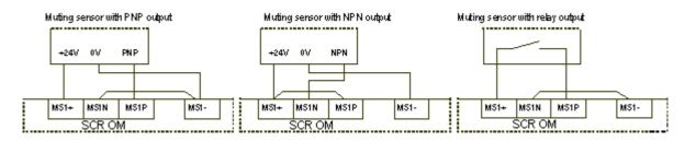
MSxP and MSxN must always be connected on the SCR OM.
