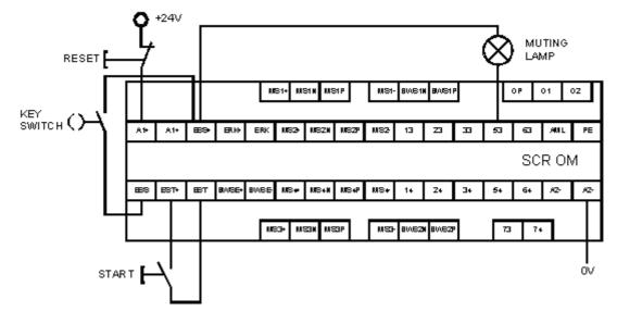
Only connect the operating voltage to terminals A1+ and A2- when the remaining wiring has been completed.
