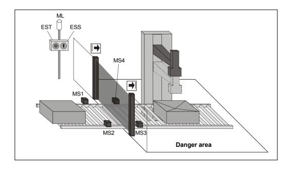
MS1, MS2, MS3, MS4 EST Muting sensors Start button ML Muting lamp ESS Key-operated switch
