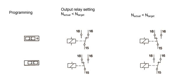
Output relay setting during time delay
