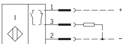
The PNP normally-open or PNP normally-closed function can be selected via an integrated switch.
