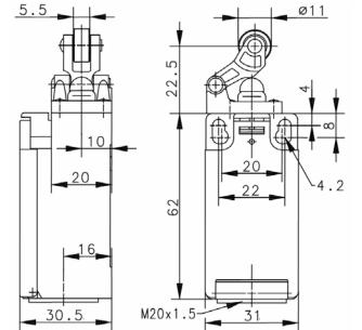
Tolerance: Operating point ± 0,25mm; Off Actuating force ± 10%
