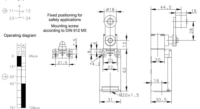
Tolerance: Operating point ± 3,5 °; Operating torque ± 10 %
