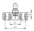
Mounting screw M5 according to DIN 912 or DIN EN ISO 4762
