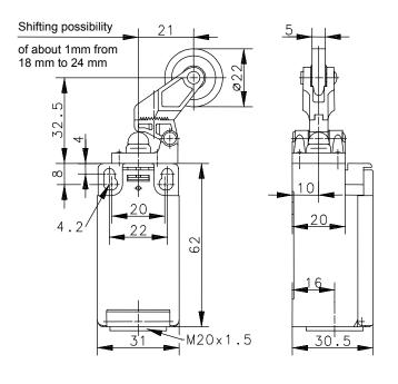
Fixed positioning for safety applications Mounting screw according to DIN 912 M5
