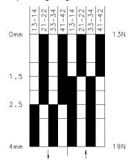
**Tolerances** Operating point: ± 0,25mm; Actuating force: ± 10% ON OFF
