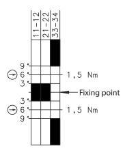
Fixing point in the range  $0^{\circ}$  ...  $270^{\circ}$  freely selectable
